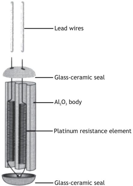
The measuring point is located at 8 mm from the end of the sensor body.
