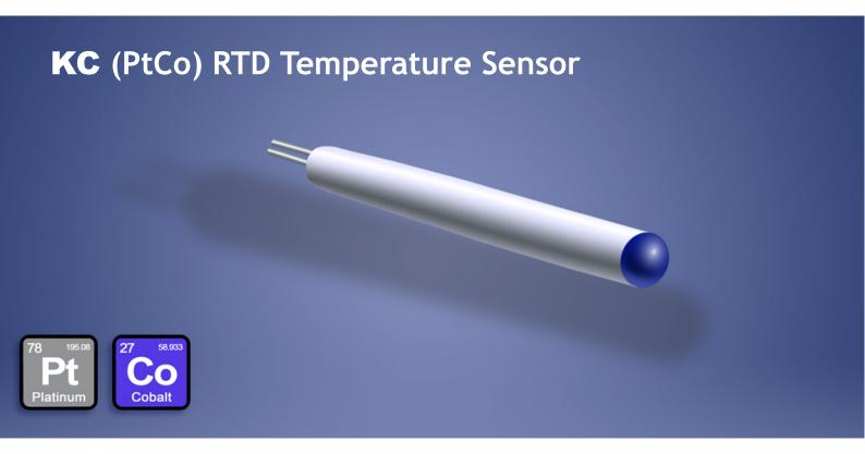
Platinum cobalt resistance temperature sensors are specifically designed for cryogenic applications. The PtCo100 element has higher sensitivity at cryogenic temperatures compared to a standard Pt100, resulting in higher resolution at extremely cold temperatures. Low hysteresis is accomplished via a highly engineered sensor coil configuration, designed to securely support the sensing wire while minimizing thermal expansion measurement errors.
